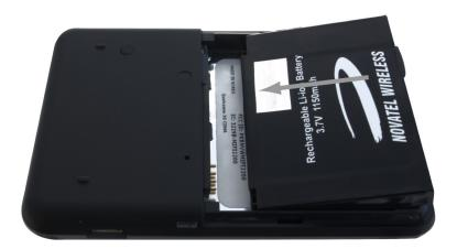
**3** Once the battery is secure, place the battery cover back on the device until the battery cover locks into place.
