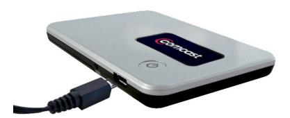
**6** Plug the other end of the AC wall charger into the appropriate electrical outlet. Charge for at least four hours.
