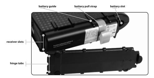
**3.** Push the battery pack into the bay until it latches into place. The following diagram shows a Telephony Modem with a 4.4 Ah lithium-ion battery pack installed. If you are taking the battery out of the unit, make sure to use the battery pull strap to dislodge the battery.
