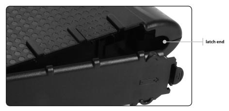
2. Hold the battery pack so that the guides on the battery align with the slots on the Telephony Modem and slide the battery into the bay. The diagram below shows the proper orientation. Batteries will not insert completely into the Telephony Modem if not oriented correctly.
