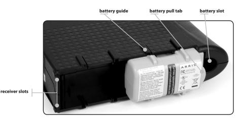
**3.** Push the battery pack into the bay until it latches into place. The following diagram shows a Telephony Modem with a 2.4 Ah lithium-ion battery pack installed. If you are taking the battery out of the unit, make sure to use the battery pull tab to dislodge the battery.
