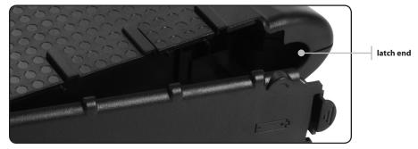
Hold the battery pack so that the guides on the battery align with the slots on the Telephony Modem and slide the battery into the bay. The diagram below shows the proper orientation. Batteries will not insert completely into the Telephony Modem if not oriented correctly.
