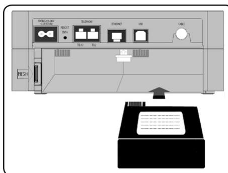
Once the battery installation is complete, plug your CDV modem back into the power outlet. Check for dial tone. The battery can take up to 24 hours to fully recharge.
