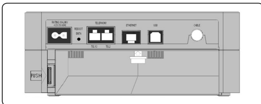
3. Insert the battery into one of the rear battery compartments, as shown in the illustration, then replace the battery cover.
