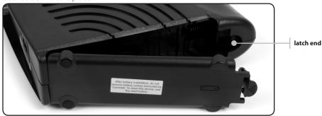
**3.** Hold the battery pack so that the guides on the battery align with the slots on the Telephony Modem and slide the battery into the bay. The diagram below shows the proper orientation. Batteries will not insert completely into the Telephony Modem if not oriented correctly.
