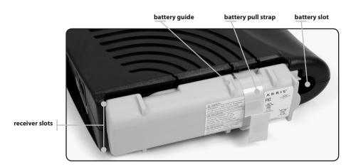
**4.** Push the battery pack into the bay until it latches into place. The following diagram shows a Telephony Modem with a 4.4 Ah lithium-ion battery pack installed. If you are taking the battery out of the unit, make sure to use the battery pull strap to dislodge the battery.
