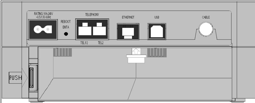
2. Insert the battery into one of the rear battery compartments, as shown below then replace the battery cover
