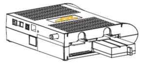
3. Push the battery into the bay until it latches into place. The following photo shows a modem with both batteries installed. Both Models only have one battery so Model TM402P should have the battery inserted in Bay 1 and Model TM402G will have the battery inserted into the available bay.
