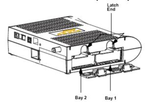
2. Hold each battery by its pull tab and insert the batteries into the bay. The photo below shows the proper orientation. Batteries will not insert completely into the modem if not oriented correctly. For Model TM402P insert the battery into Bay 1. Model TM402G has only one Bay.
