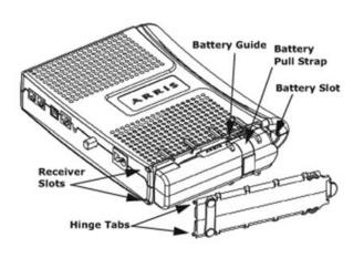
3. Push the battery pack into the bay until it latches into place. The following diagram shows a modem with a battery pack installed. If you are taking the battery out of the unit, make sure to use the battery pull strap to dislodge the battery.
