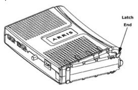
2. Hold the battery pack so that the guides on the battery align with the slots on the modem and slide the battery into the bay. The diagram below shows the proper orientation. Batteries will not insert completely into the modem if not oriented correctly.
