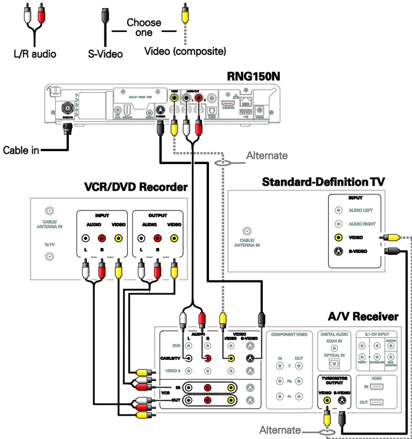
*Note: Solid lines indicate optimum connections.*
