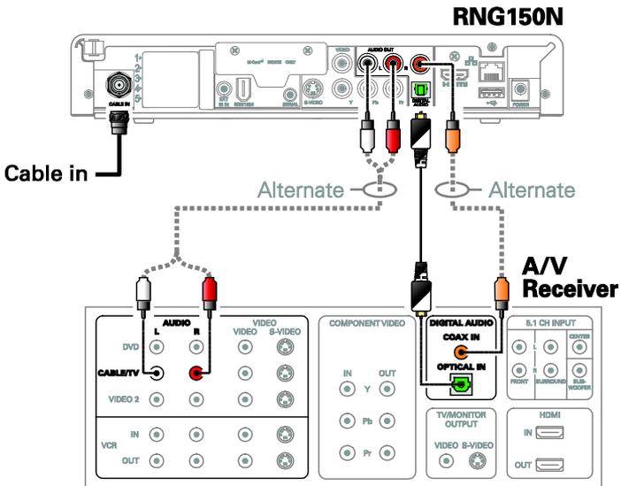
*Note: Only (1) audio connection needs to be made to an A/V Receiver.*
