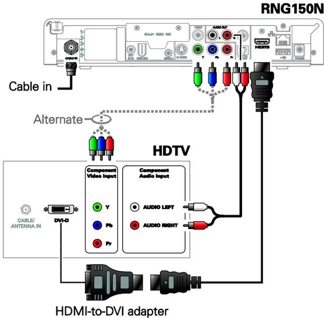
*Note: Only (1) video connection and (1) audio connection needs to be made to an HDTV.*
