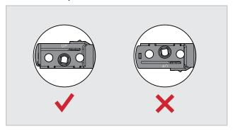
Reinstall the latch, making sure the word "UP" faces upward.
