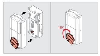
Reinstall the interior assembly on the door, and reinstall the battery pack.
