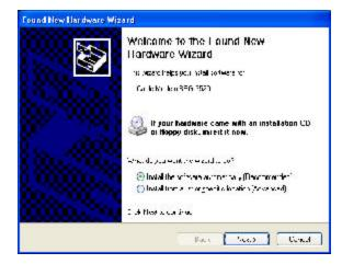
**2** Select *Install the software automatically* (Recommended) and click *Next.* Note: This installation will complete automatically.
